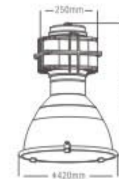
Type: NH001/250W Lamp: OSRAM HQI-E250W/D I max = 3579.01cd
