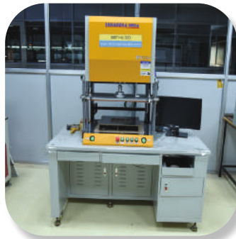
BBT BBT is a process used for testing PCB circuit
