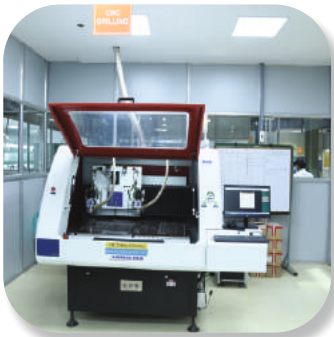
CNC CNC is a process for drilling and routing
