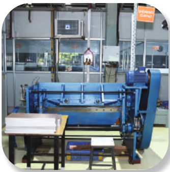
SHEARING Shearing is a process where sheet cutting is done according to PCB size
