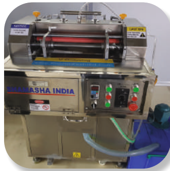
V-CUT Depanalization for break pcb
