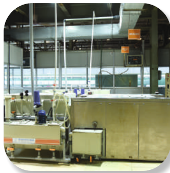
BRUSHING Brushing is the cleaning process after cutting
