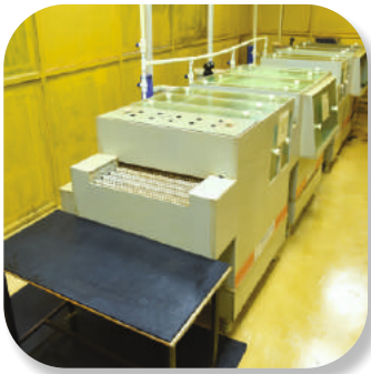
ETCHING In etching it removes excess copper, ink stripping and removing ink from printed circuit
