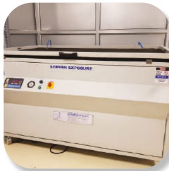
EXPOSING Exposing film for Circuit, Masking & Legend
