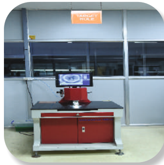
TARGET HOLE It's a guide hole for printing and CNC
