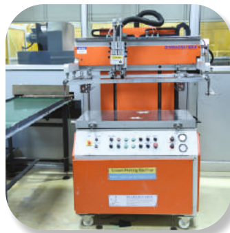
PRINTING There are three types of printing, Circuit printing, Masking printing & Legend printing
